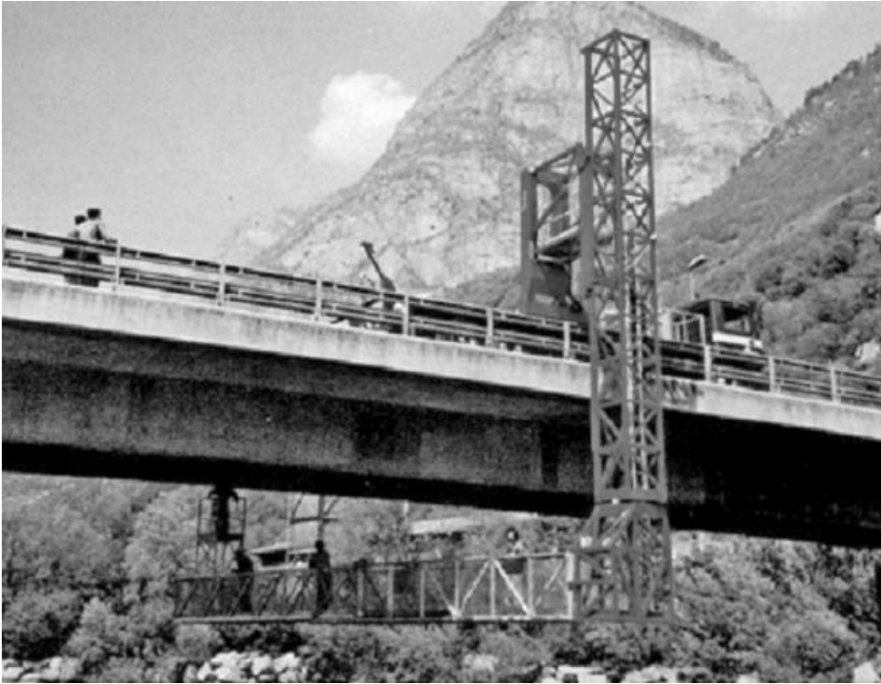
Figure 3.5 Bridge inspection unit (reproduced courtesy of MOOG GmbH, copyright reserved)
