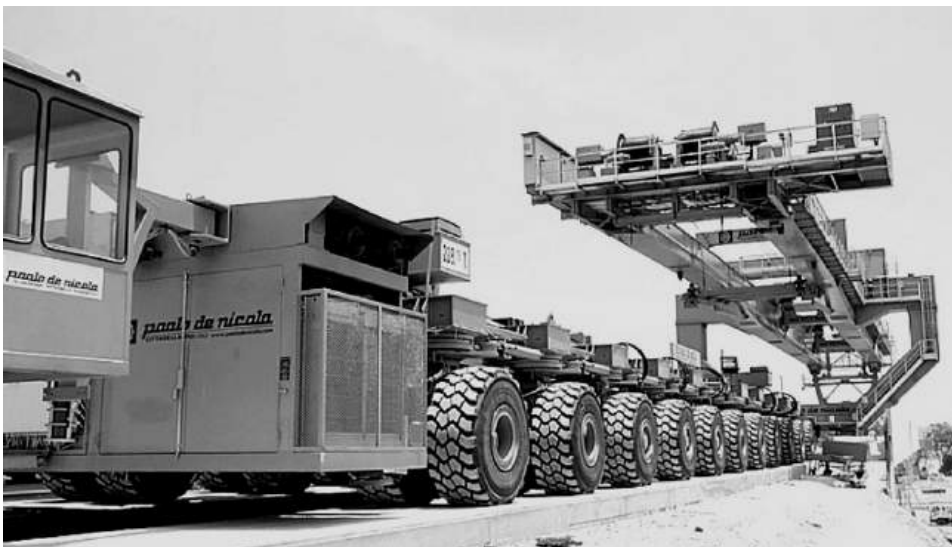
Figure 14.10 Beam transporter (reproduced courtesy of Tony Gee and Partners LLP, copyright reserved)
