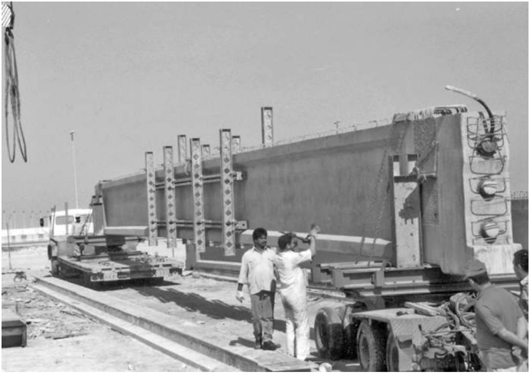
Figure 10.19 Beam transporter (reproduced courtesy of Hyder Consulting (UK) Ltd, copyright reserved)
