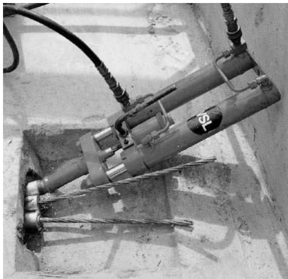
Figure 2.12 Jack for stressing single strand (reproduced courtesy of VSL International, copyright reserved)
