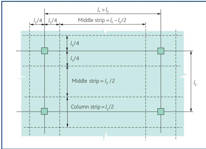
At internal columns, unless rigorous serviceability calculations are carried out, top reinforcement of area  $0.5 A_t$  should be placed in a width equal to the sum of 0.125 times the panel width on either side of the column.  $A_t$  represents the area of reinforcement required to resist the full negative moment from the sum of the two half panels each side of the column. It is also advisable to apply this requirement to perimeter columns as far as is possible.
